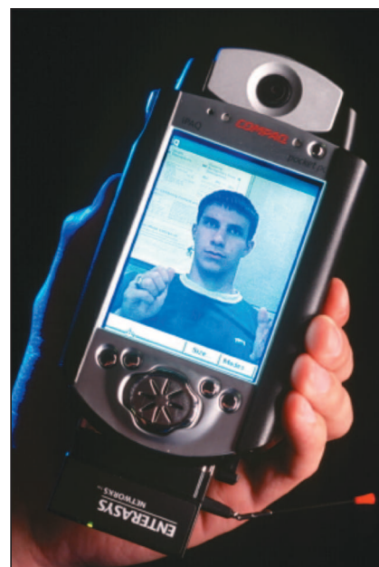
Figure 1. The commercial iPAQ with BackPAQ, jointly developed by Compaq Research Labs and MIT. The BackPAQ contains a video camera, an accelerometer, a microphone and headphone connectors, and two PC card slots.
