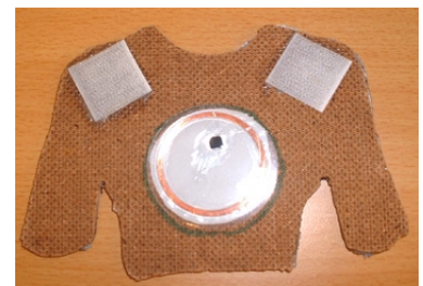
Figure 2. The rear side of a clothes piece showing the RFID tag and Velcro.
