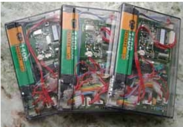
Figure 2: Smart-Its assembled in a cassette box.
