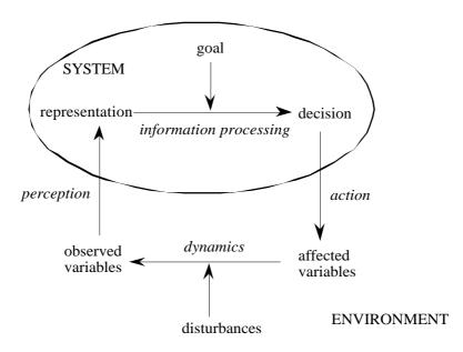
Fig. 2: basic components of a control system
