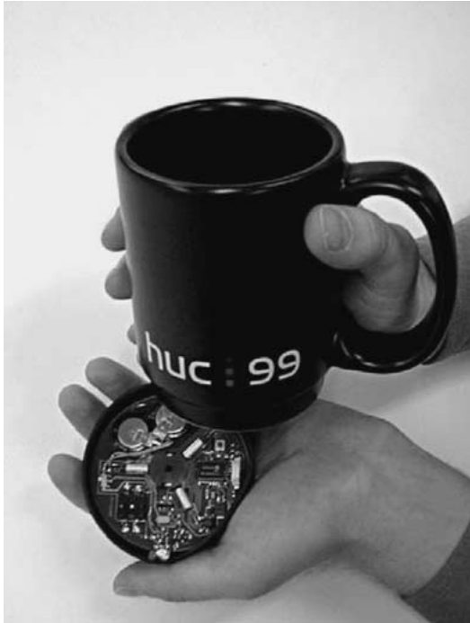
Figure 4. The Mediacup is an ordinary coffee cup with sensors, processing and communication embedded in the base.
