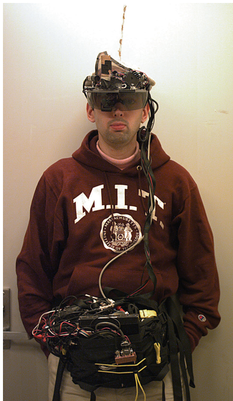
The author and his wearable multimedia computer/personal visual assistant. The apparatus includes a miniature computer screen and sensor array in the eyeglasses, Internet connection, and a multimedia computer with special-purpose video processing hardware.
