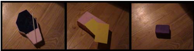
Figure 1: mock-up of a) a Pocket PC, b) magnetic tag reader, c) small sensor box
